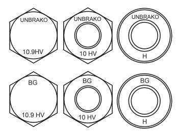
Note - The 10.9 HV & 10 HV means that the product was manufactured to BS EN 14399-4.
