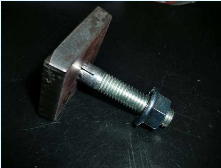
Figure 2.3 Complete tension test; pull-through
